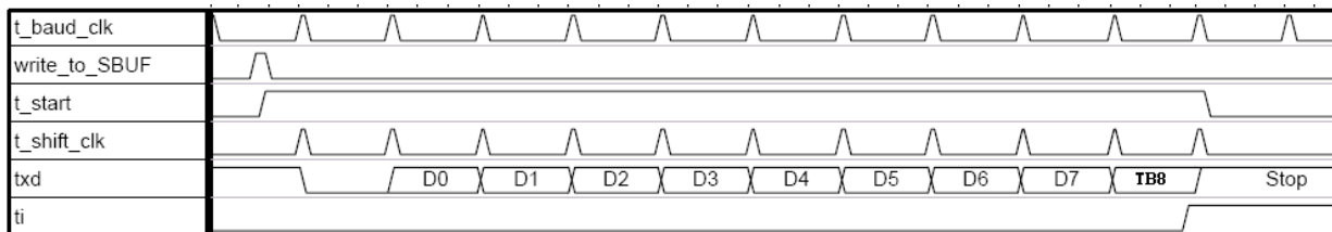
Fig. 8-5: Transmit modes 2 and 3 for Serial 0
