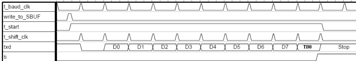
Fig. 8-5: Transmit modes 2 and 3
